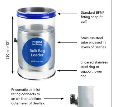
**NOTE:** If using in Atex Dust Zones, the up-line pipework and pneumatic air-line inlet fitting should be earthed.
